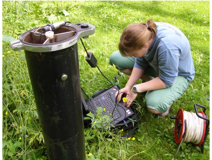
The UTRCA's Monitoring Technician downloads water level data from a groundwater monitoring well.
